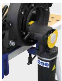
Including second saw blade position to cut off tube elbows
