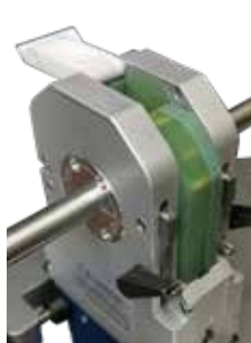
Flip up weld head cover "Flip Cover"
